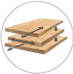
Roof (CTL) Construction
