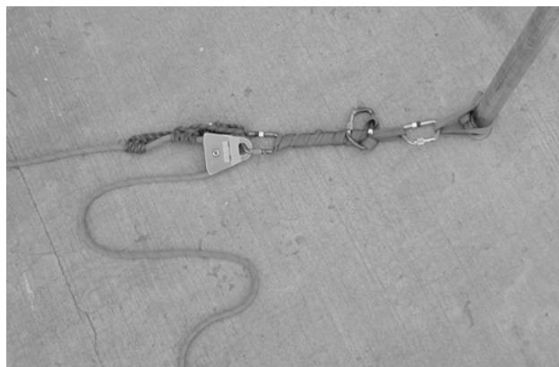
Figure 15.2 Tandem Prusik Belay with Prusik Minding Pulley
