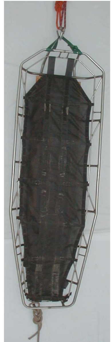
Figure 13.9 Litter Rigging, Vertical Raise
