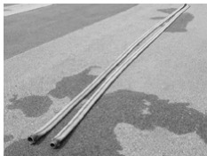
Step 1: Lay the hose flat and bring the coupling alongside each other.
