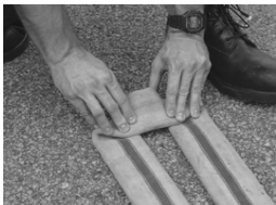
Step 3: Fold the far end over and roll toward the couplings, creating a double roll.
