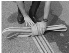
Step 4: From the point where the hose crosses, begin to roll the hose toward the couplings with the loop as its center. This creates a loop on each side of the roll.
