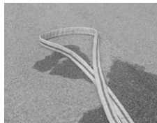
Step 2: Move one side of the hose over the other creating a loop. This loop creates the carrying shoulder loop.
