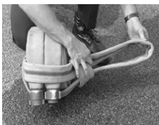
Step 6: Position the loops so one is larger than the other. Then pass the larger loop over the couplings and through the smaller loop.
