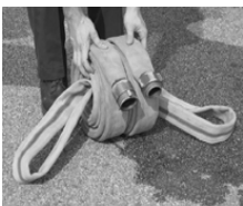
Step 5: On completion of the rolling, position the couplings on the top of the rolls.
