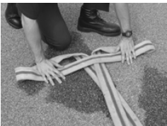
Step 3: Bring the loop back toward the couplings to the point where the hose crosses.
